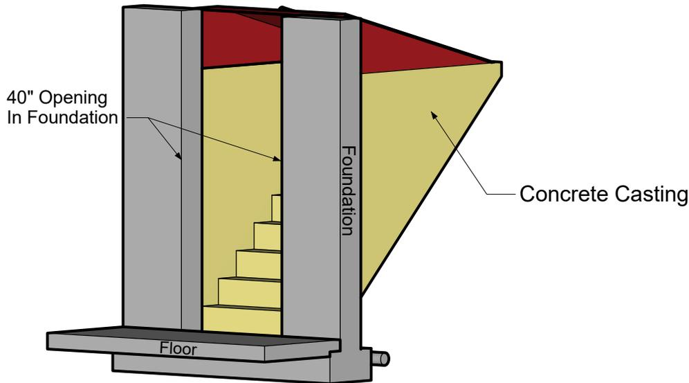
Note: Concrete Casting Size is measured from the Top of Footing to Finished Grade
